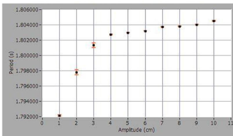
Within the necessary bounds of 4-6cm the starting amplitude of 4cm was selected as best since it had a low uncertainty, represented by narrow error bars, and lied most securely in the region of amplitude-period independence.
